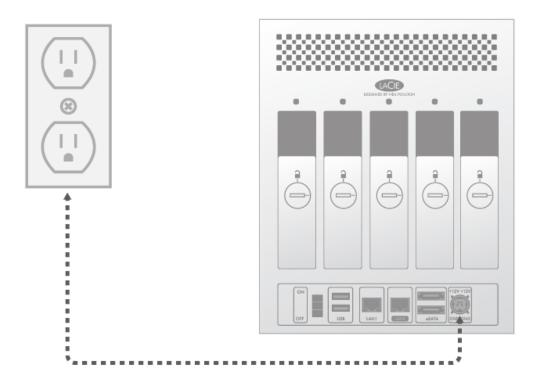
2. Turn the device on via the power button on the back of the enclosure.
