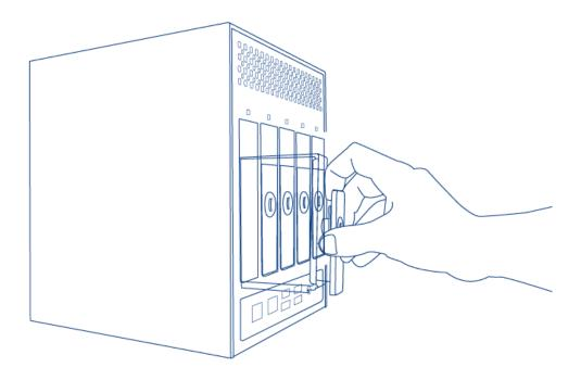
4. Repeat the process if you are adding more than one disk. Make certain to remove the Disk Trays in the proper slot order.
