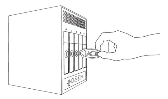
2. Draw out the drive tray by inserting your finger into the space behind the drive tray handle and pulling to disengage the drive.
