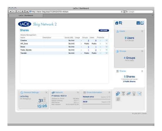
Shares—network folders—comprise the storage capacity of your LaCie NAS. Out of the box, it has two shares, Share and Public, and USBShare (d2/2big only) or iSCSIShare (5big only) is created automatically when storage is allocated to it using the Dashboard. The Shares page in the Dashboard allows the administrator to assign quotas and access rights to users and groups, and to toggle share-level service activation.
