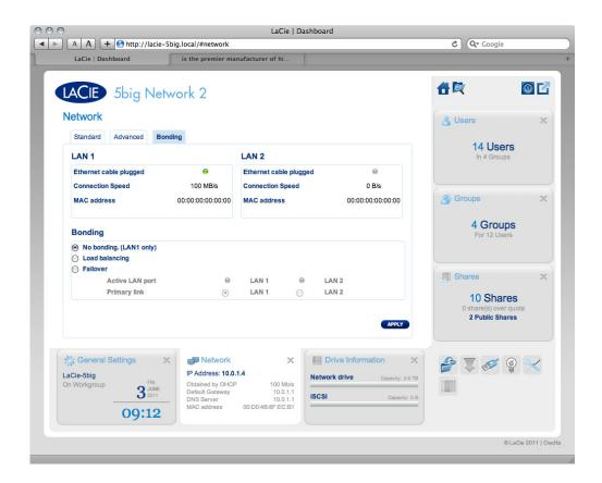
This section displays features made available to the 5big Network 2 when it is connected to the network via two Ethernet cables. In the first two boxes, information about LAN1 and LAN2 are displayed.
