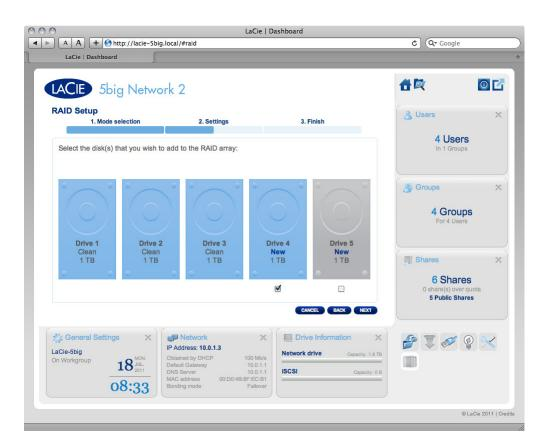
3. Choose a RAID level, then click **NEXT**. Note that you can choose to add the new disk as a spare. If you leave a disk as a spare and one of the disks in the array fails, the array will automatically be rebuilt using the spare. This method assures continues data access even in the case of disk failure, but doesn't allow you to use the capacity of the spare disk.
