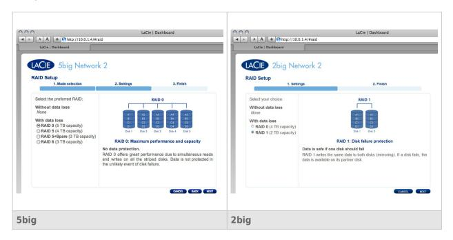
If you select a RAID mode under the heading **Without data loss**, converting the new mode will not erase files stored on your LaCie NAS. If you select a RAID mode under the heading **With data loss**, converting to the new mode will erase files on the shares (but Dashboard configuration will not be affected).
