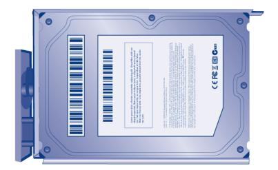
3. Using the Phillips head screwdriver, carefully fasten all four screws into the four tray slots. Do not overly tighten the screws. Doing so can affect the integrity of the screw holes on the drive as well as the threads on the screws.
